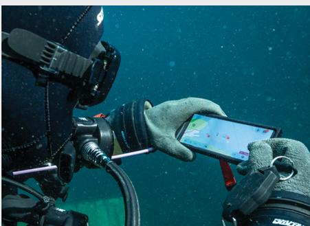
Diver consoles enable diver-to-diver communication with position tracking and short messages exchange.
