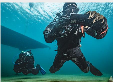
A diver tracking buoy with built-in GNSS and WiFi provides a bidirectional link from land or a support vessel to divers equipped with lightweight trackers based on compact EvoLogics 18/34 modems.
